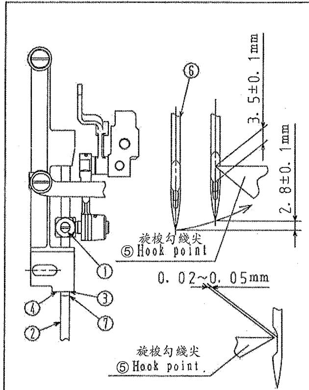
◇Adjust the timing between the needle and the hook as follows
